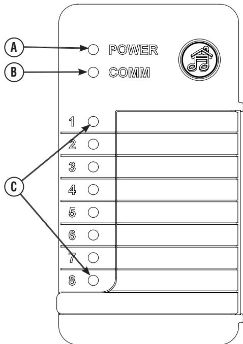
A decal is provided that can be labeled with the managed appliances/loads and placed next to each priority LED.
