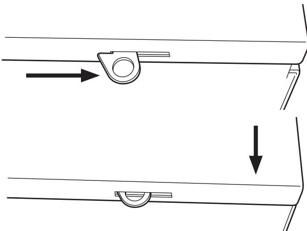
To close and latch door, push door closed against enclosure. While in this position, push door upwards. This will cause spring-load door lock to engage and latch door in place. Enclosure door MUST be closed and latched at all times except when system is being serviced.
